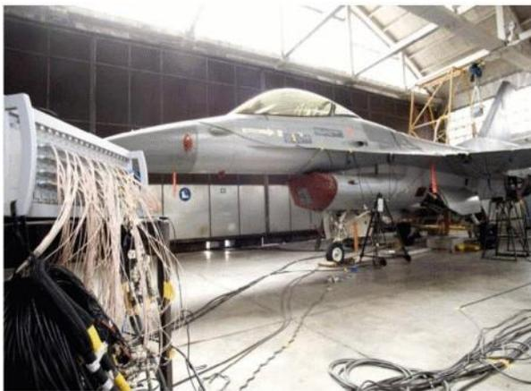
Fig. 6 – Test bench per flutter
